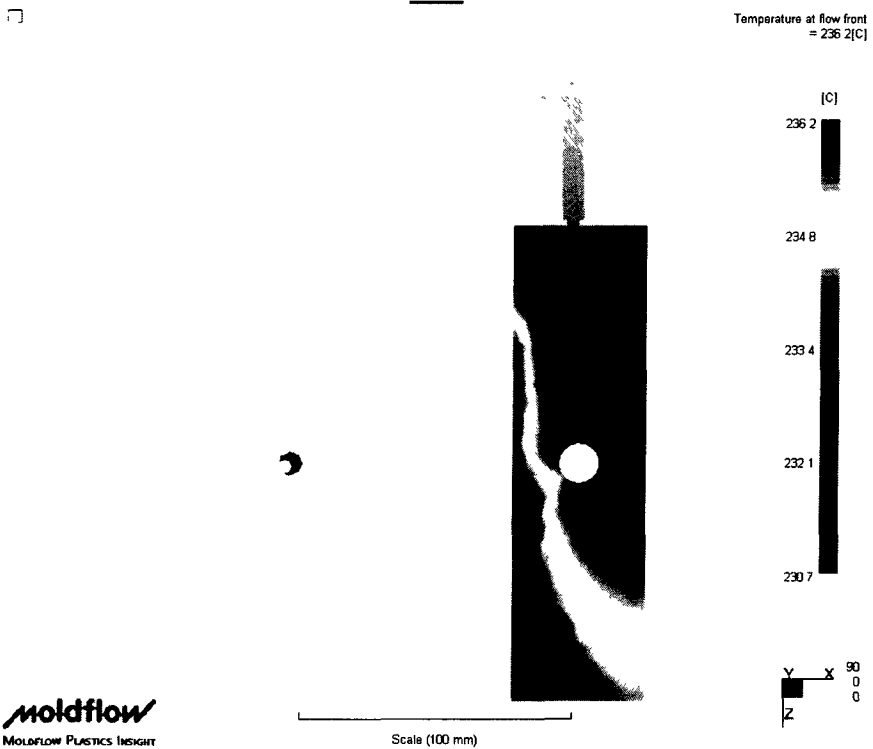
Figure 8d - Temperature at flow front in obstacle pin cavity, mtl: CR4500 @ 6.3 cc/s
